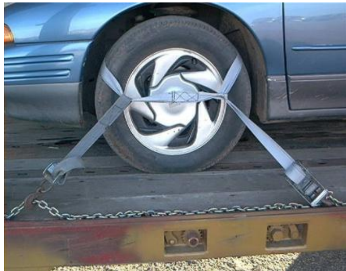
Figures 2 and 3: One point and two point soft-ties – NOT permitted
