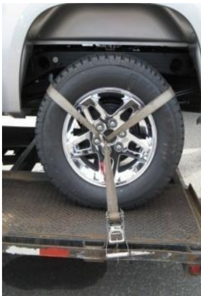
Figures 2 and 3: One point and two point soft-ties – NOT permitted
